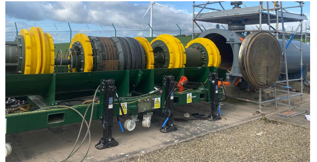
Remote Tecno Plug insertion, courtesy of STATS Group
