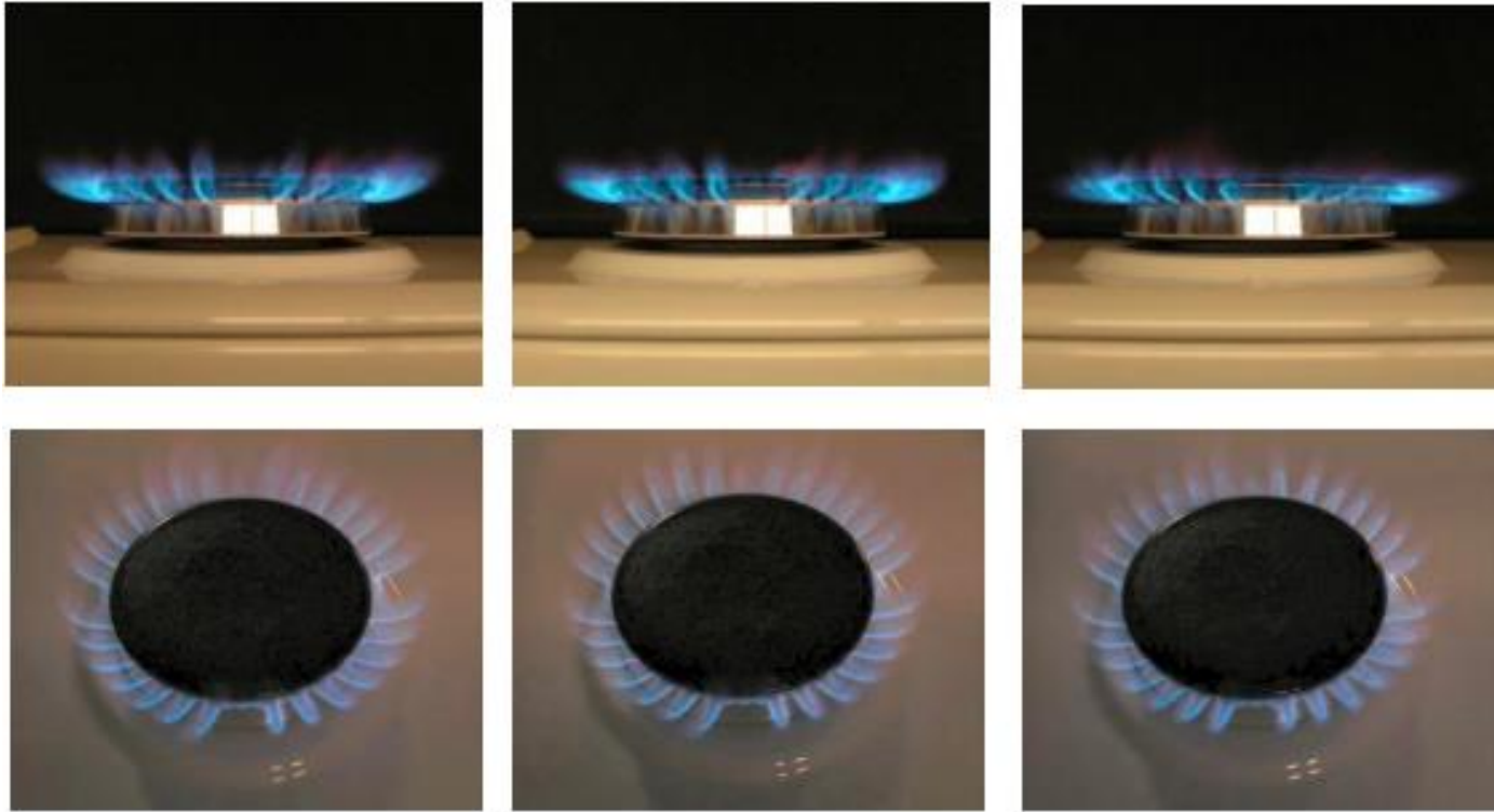
Figure 6 Gas ring fuelled by hydrogen enriched natural gas (62), hydrogen content of gas increasing from left to right
