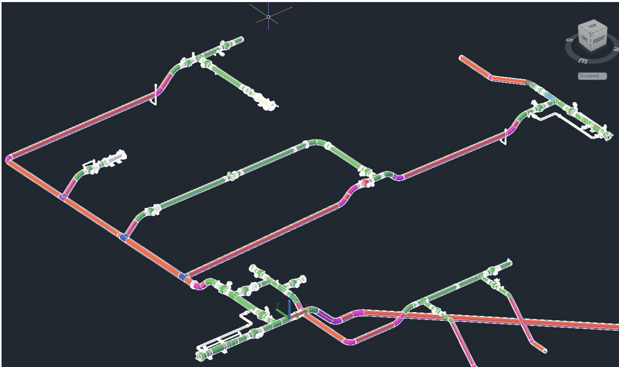
Figure 27: Pannal AGI Pipework with PIE GRAID Model Condition Colour-Coding Example 1
