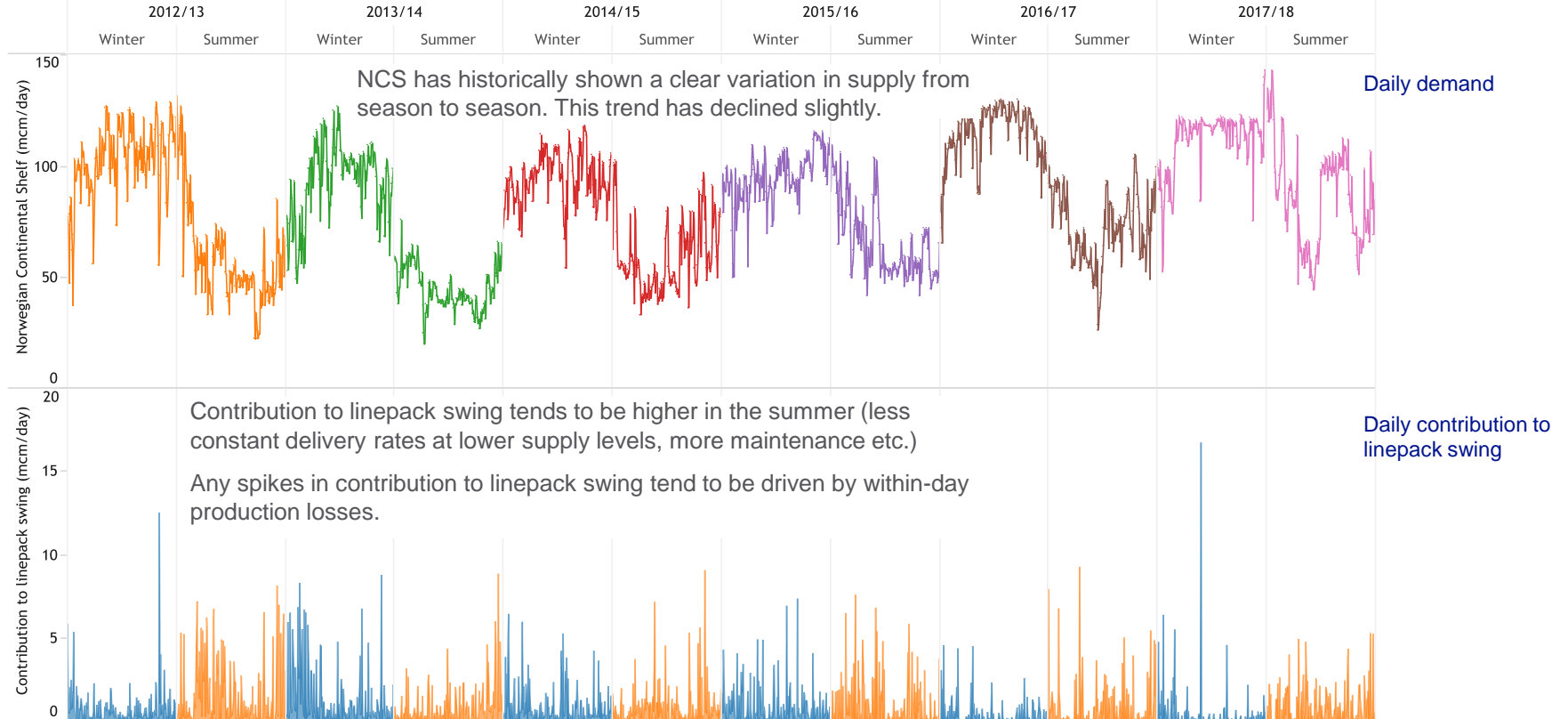
Daily NCS supply and contribution to linepack swing
