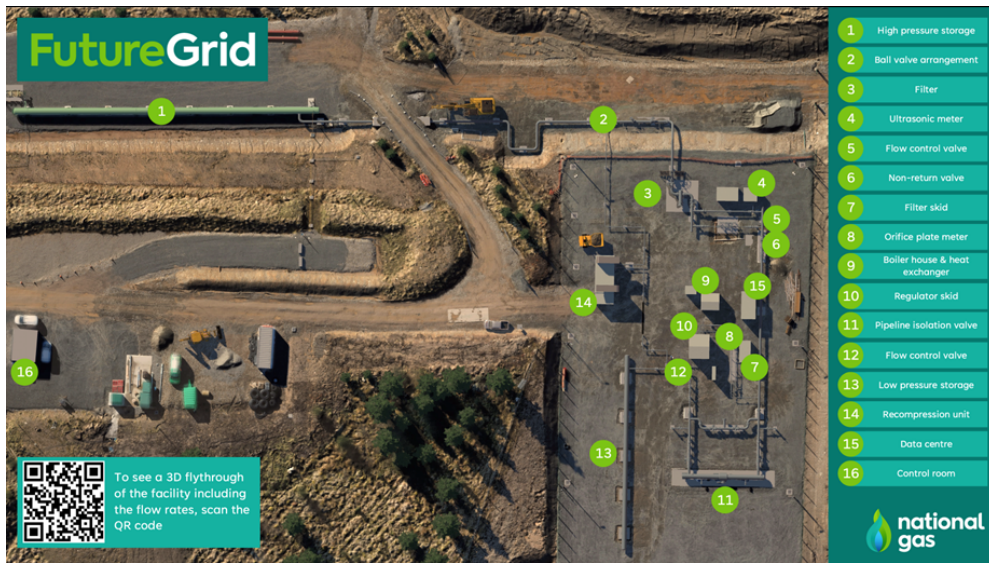
Figure 18 - Digital representation of FutureGrid from CVDT project showing each asset on the system and providing an overview of the site
