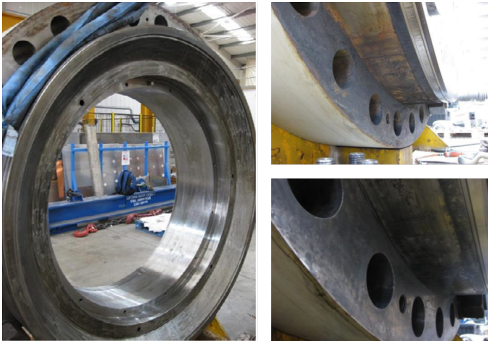
Figure 46 – Aberdeen Unit A Casing: (Top right) Rust and corrosion identified bottom half part of the outer flange of the compressor cartridge. (Bottom right) This was removed as much as possible to make correct assembly possible.
