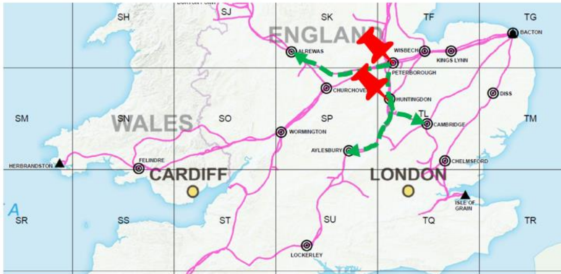
Figure 19: Importance of Peterborough and Huntingdon to the Midlands Axis - Enabling high LNG flow from Milford Haven to Bacton for exporting to or importing from Europe
