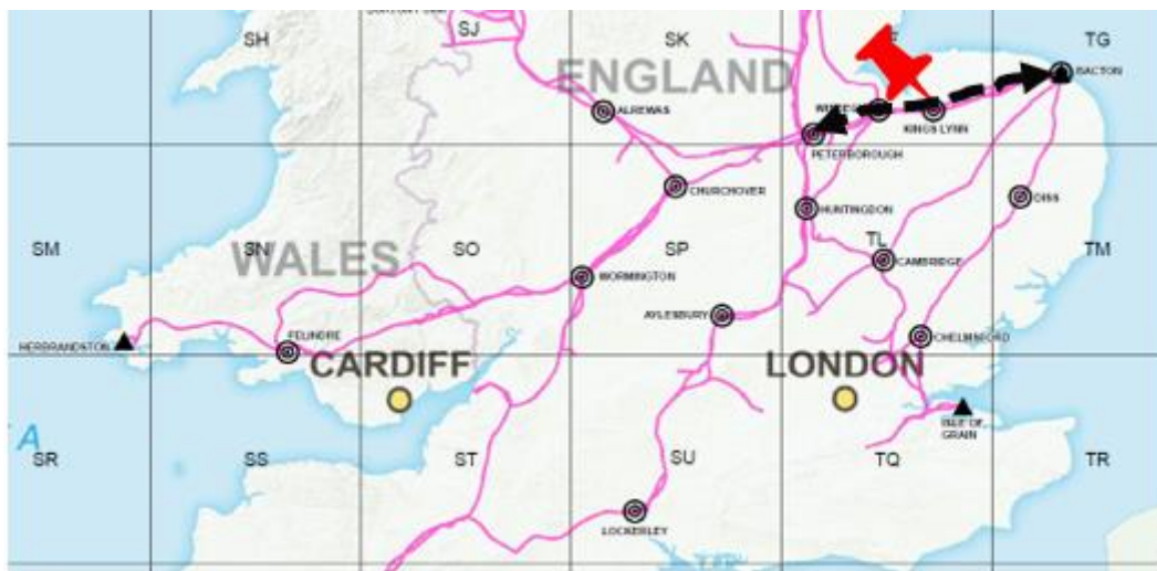
Figure 30: King’s Lynn’s role in the Midlands Axis – Enables flow from LNG terminals at Milford Haven to Bacton for export to and import from Europe
