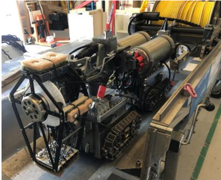
Figure 41: GRAID robotic platform and tether reel following the innovation project
