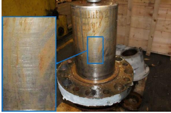
Figure 2: Leaking stem due to wear
