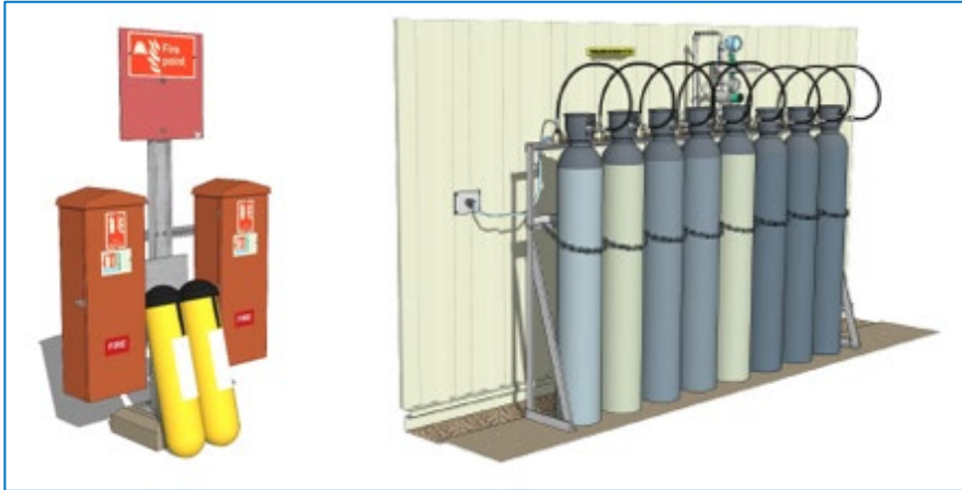
Figure 7: Cabs Fire Suppression (Fire point and Pressurised nitrogen bottles for HI-FOG® system)
