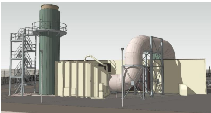
Figure 7: Compressor cab with SCR fitted
