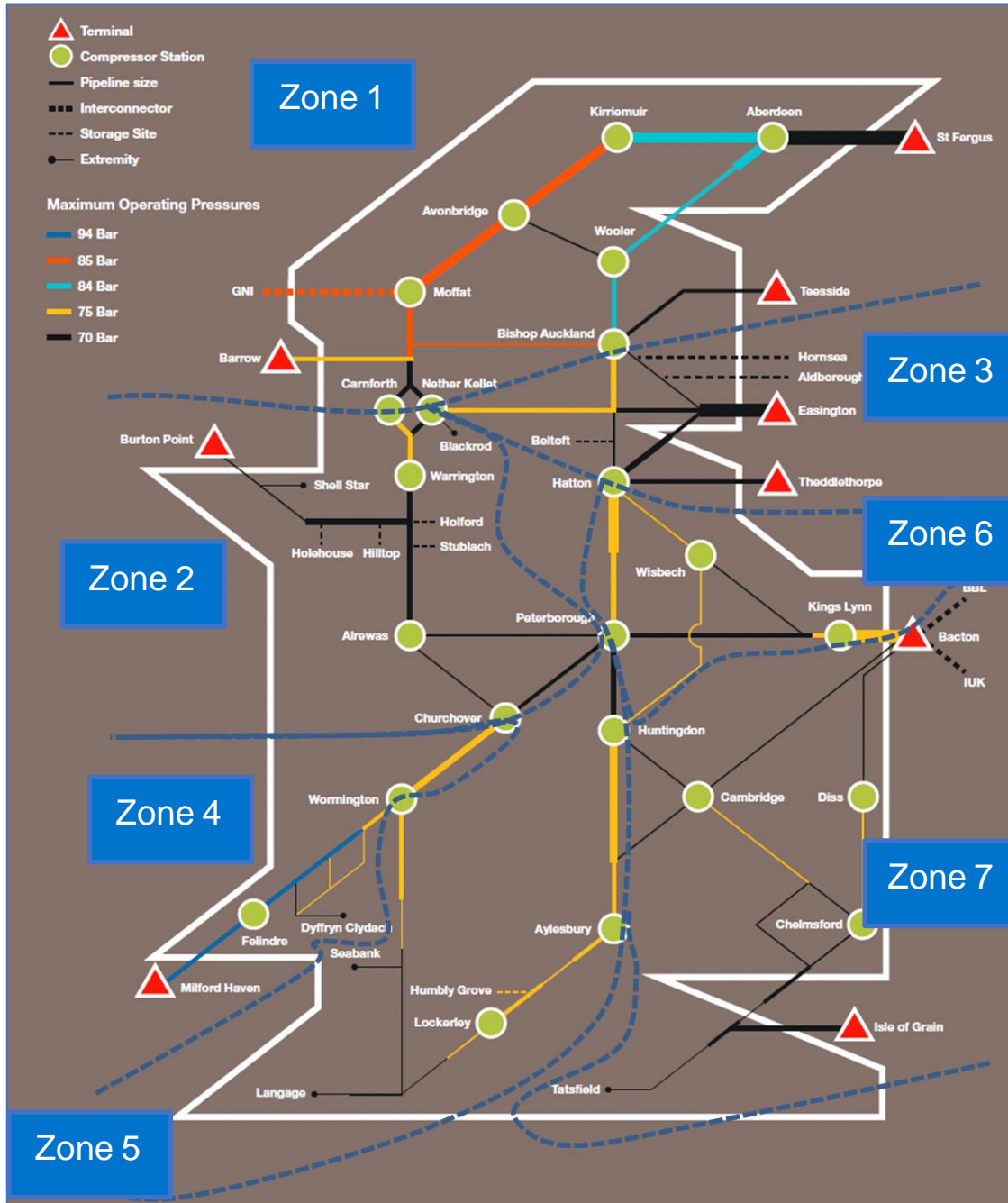
Figure 3 Gas network zones used in network capability analysis 6
