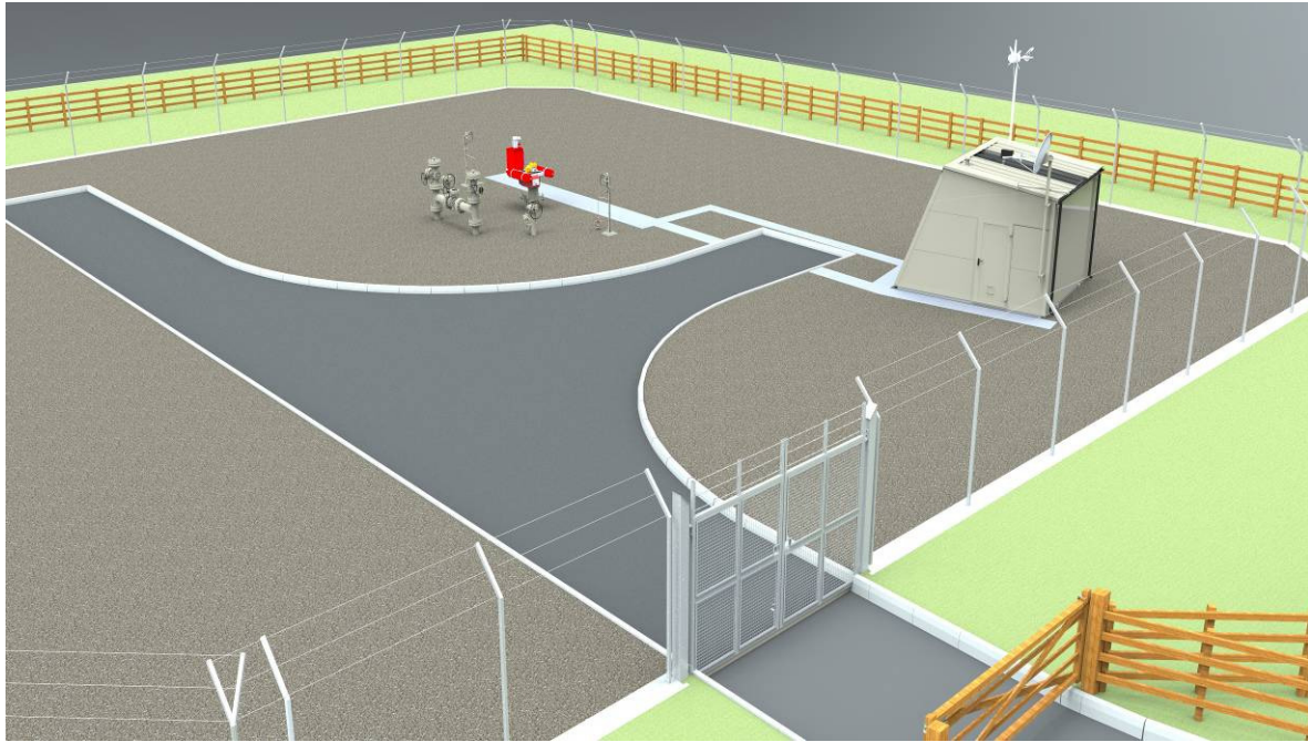
Figure 2 - Typical Block Valve Site – Consists of Standard Assemblies
