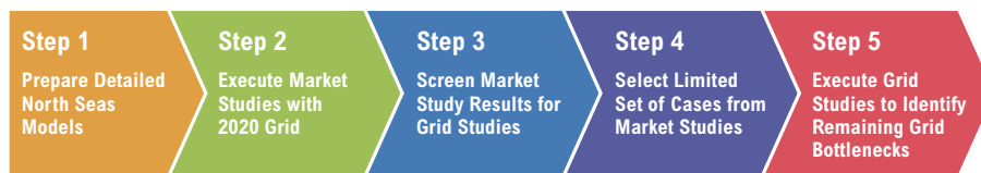
Figure 5: RG NS Methodology for calculation of Bottlenecks
