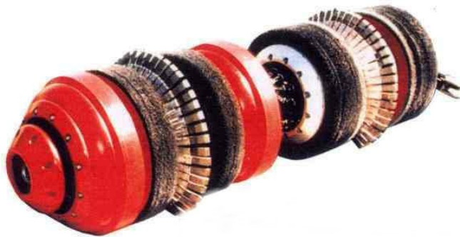
Figure 5.8 - Intelligent Pipeline Inspection Gauge (PIG)
