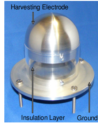
Demonstrator hardware for capacitive energy harvesting demonstrator to power a wireless sensor
