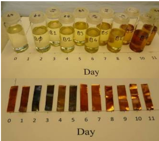
Progressive change in colour of copper strips with ageing in oil at 150°C
