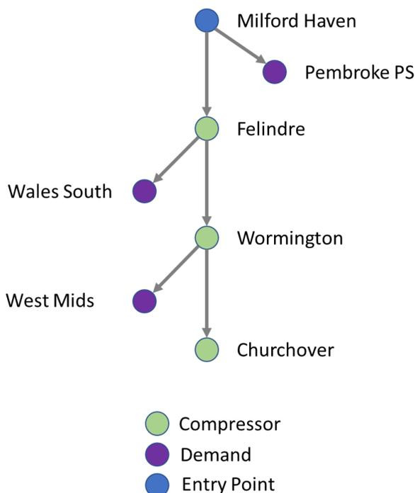
Figure 1: Schematic representation of the key NTS assets that have an influence on Milford Haven Entry capability
