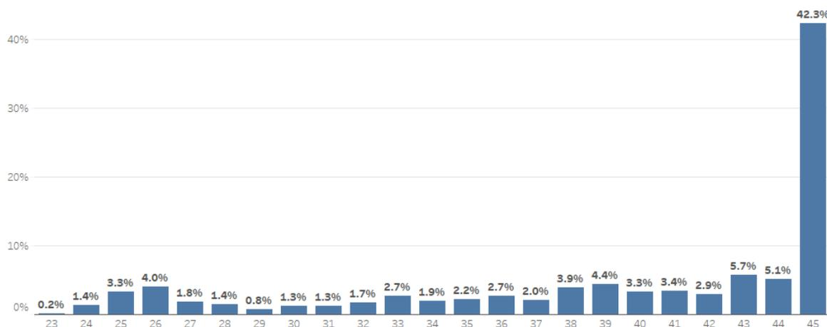
Figure 2: Overview of recent flow rates through Churchover Compressor. The figure identifies 45 mcm/d as the maximum achievable flow. N.b. Churchover Unit D used as the alternative unit will be on outage over the summer period
