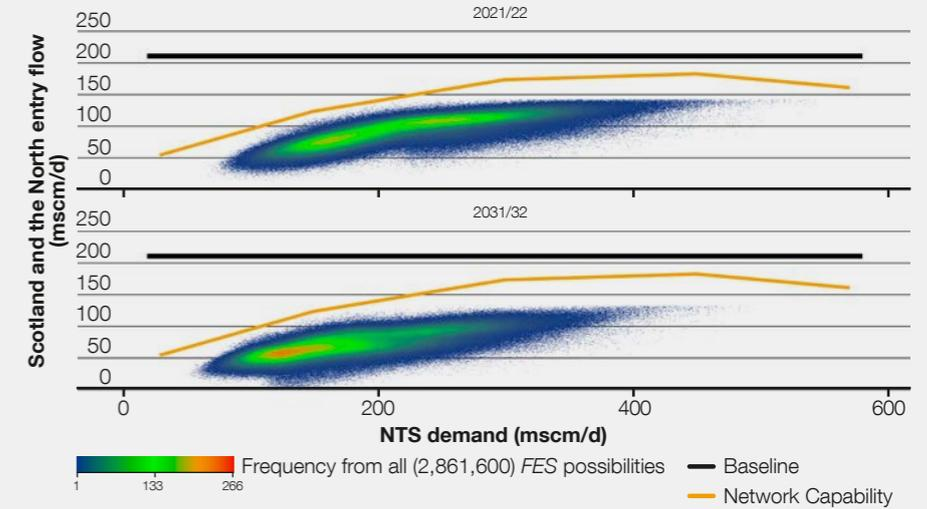
Figure 2.3 shows that we have sufficient entry capability in the zone over the next 10 years.
