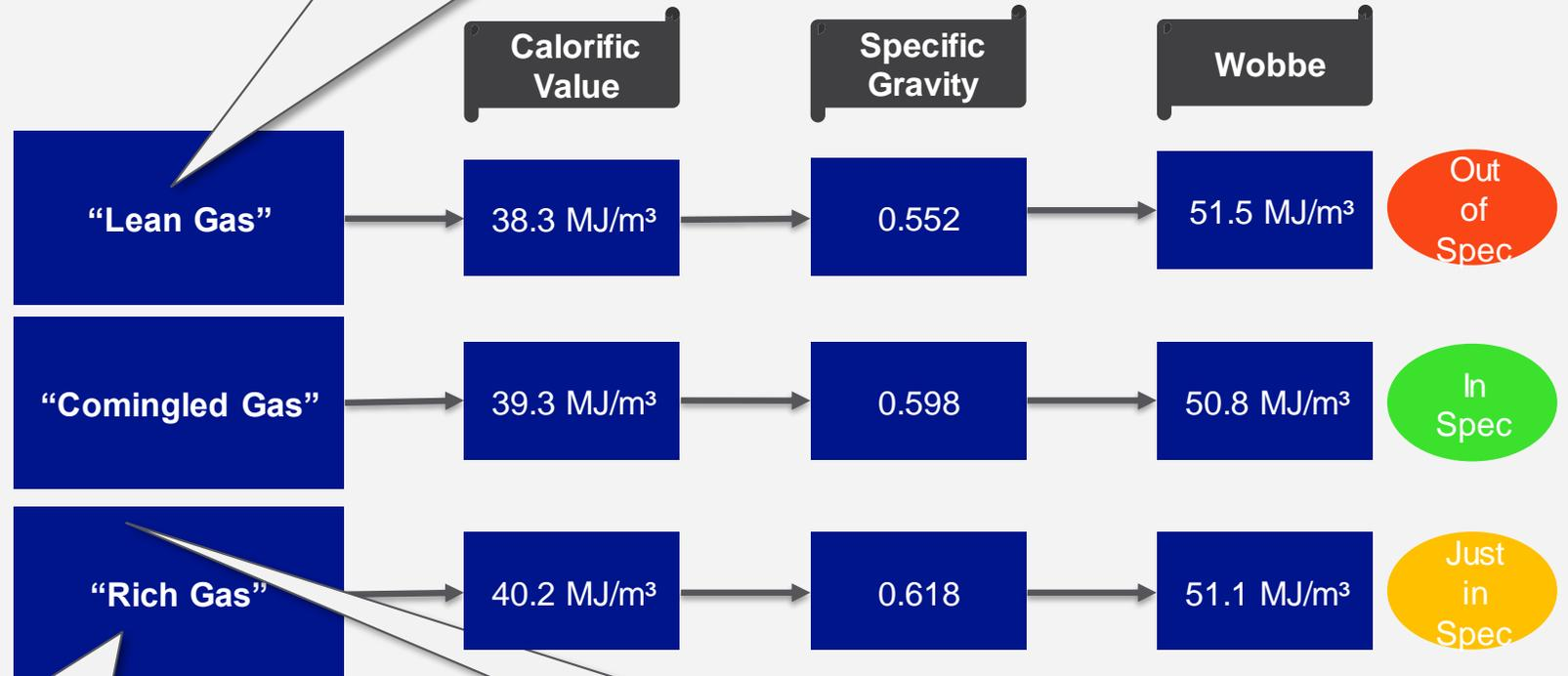
“Rich gas”, contains more larger molecules which causes a higher CV and specific gravity, nearly resulting it to fall out of the allowed Wobbe range
