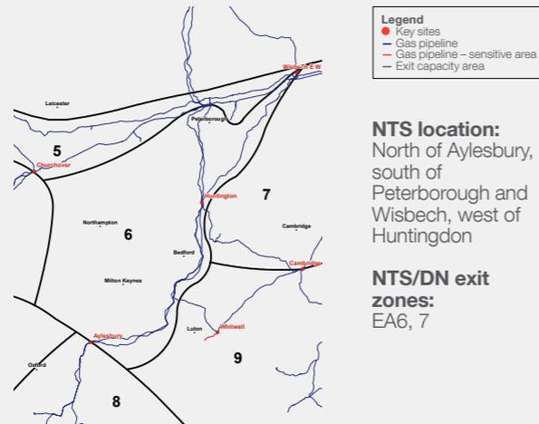
Capacity availability is sensitive to demand increases downstream in region 10, the South West. The quantity of unsold capacity indicates limited scope for exit capacity substitution from the single offtake in the region, but there may be scope for substitution from the Southern region downstream of Aylesbury. Potential non-Planning Act reinforcements could be carried out to release capacity.
